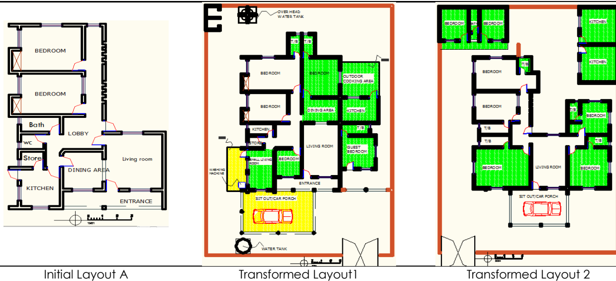
Figure 2 Illustration of a two roomed apartment with two samples of user initiated transformation.
