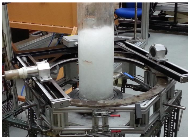
Figure 7 GammaSpider uses to study hydrodynamic behaviour of gas-water in a bubble column
