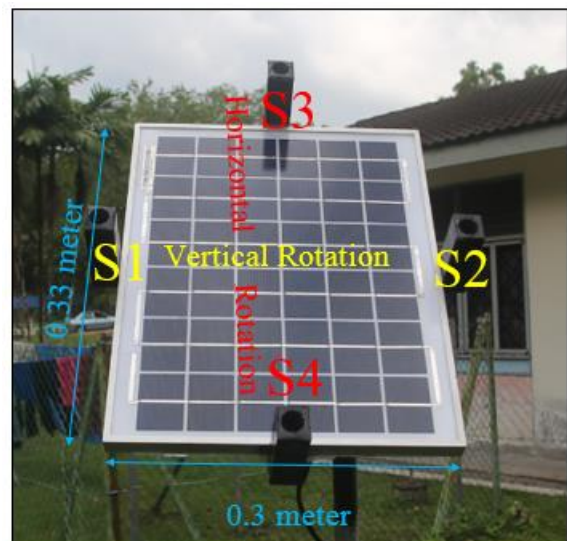
Figure 13 LDR Sensor Position on Solar PV Panel
