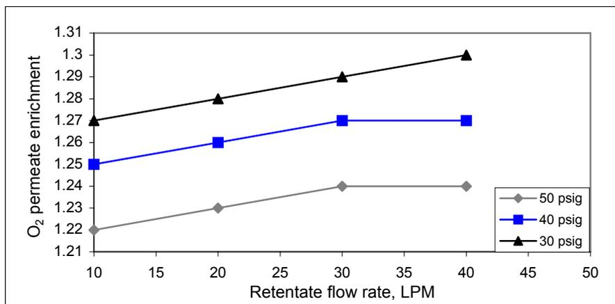
**Figure 4** O<sub>2</sub> permeate enrichment versus retentate flow rate
