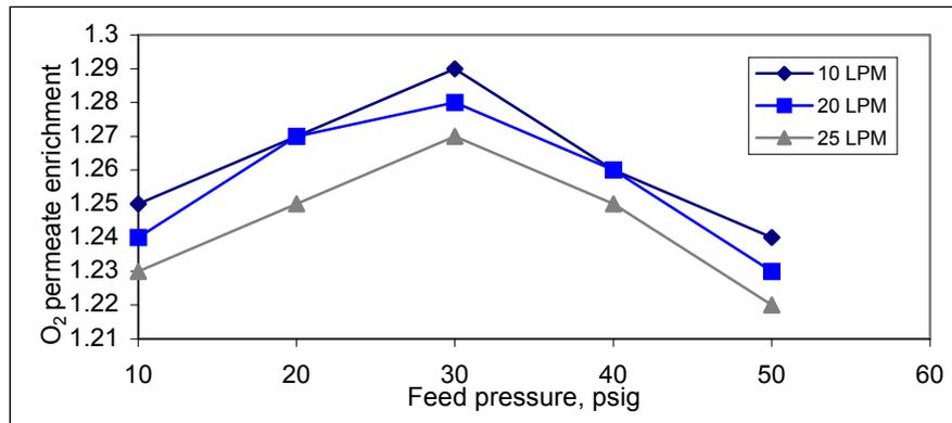
**Figure 3** O<sub>2</sub> permeate enrichment versus feed pressure
