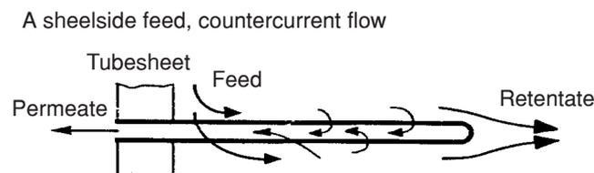
**Figure 2** Shell side feed, countercurrent flow membrane module
