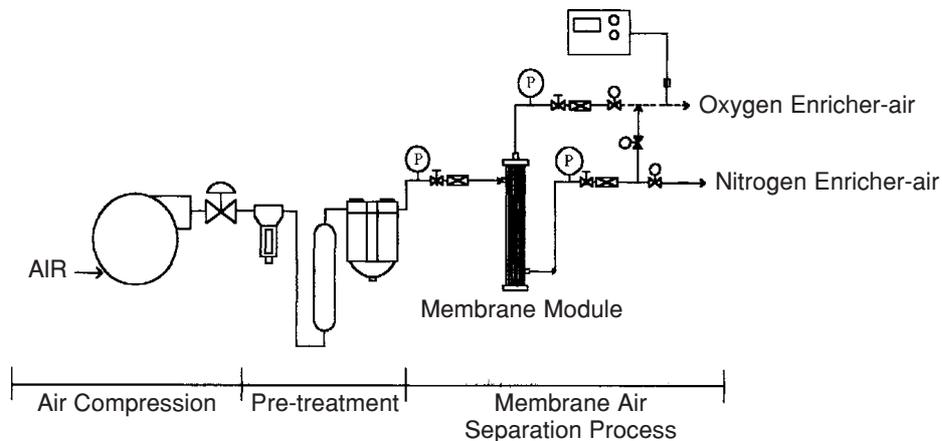
**Figure 1** Schematic system flow diagram
