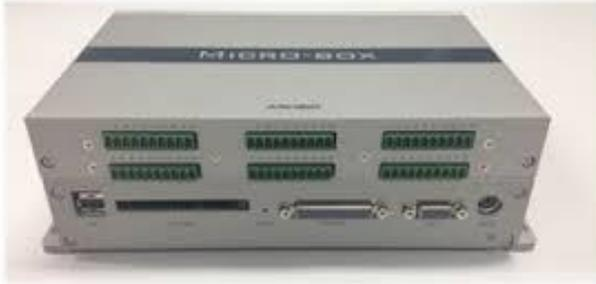
Figure 3 Micro-Box 2000 x86 Based Real-Time System
