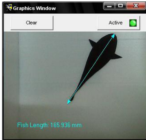
Figure 12 Prototype fish is measured repeatedly at fixed distance
