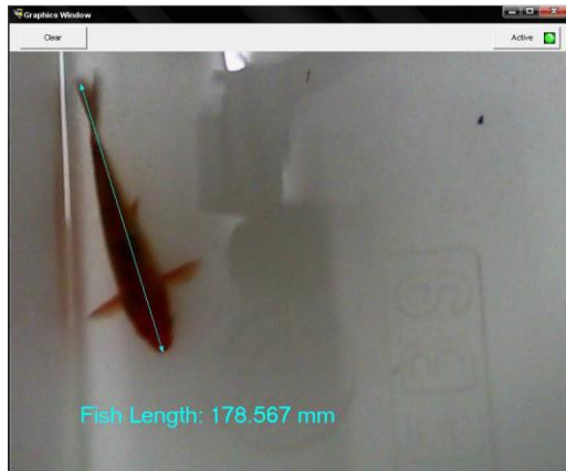
Figure 14 Length measurement on real fish at 40cm capturing distance
