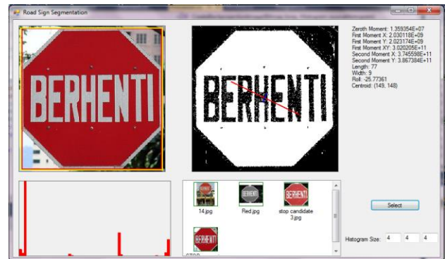
Figure 3 A red STOP sign transformed into binary image
