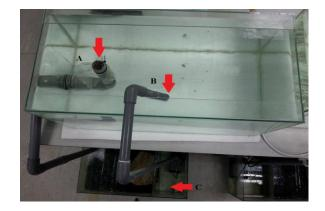
Figure 3 Glass aquarium used for observing the behaviour of phyllidiid species: A. The outlet; B. The inlet of filtered sea water; C. Filtration system
