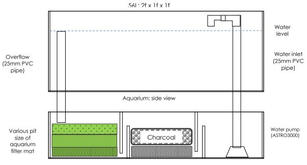
Filtration tank: side view Figure 2 Side view of aquarium setting
