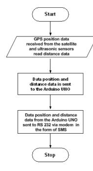
Figure 7 Position and height data sending through Wavecom Fastrack modem flowchart
