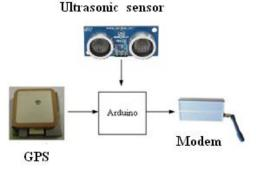
Figure 6 GPS transmitting system and ultrasonic sensor through Wavecom Fastrack modem.
