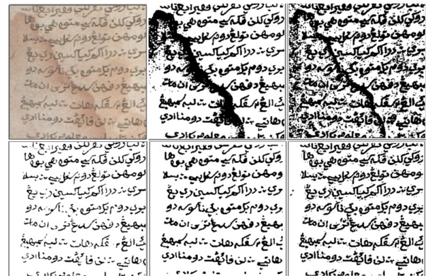
Figure 10 Cropped original and binarised document images samples (from top left to right: original document, Otsu image, Niblack image, Sauvola image, Lu image, and Su image)
