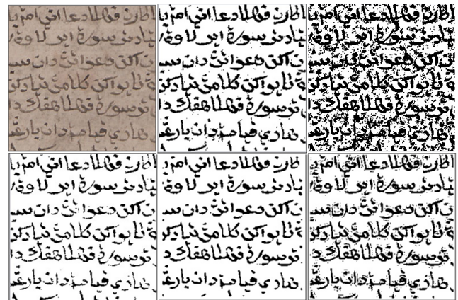
Figure 17 Cropped original and binarised document images samples for fox degradation type (from top left to right: original document, Otsu image, Niblack image, Sauvola image, Lu image, and Su image)
