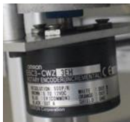
Figure 9 Omron rotary encoder attached to BLDC motor's pinion shaft
