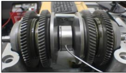
Figure 8 Position of the force sensor between the pulley sheaves
