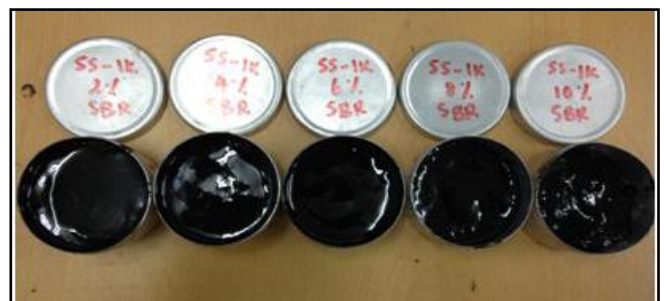
Figure 3 Samples of polymer modified emulsion (SBR)
