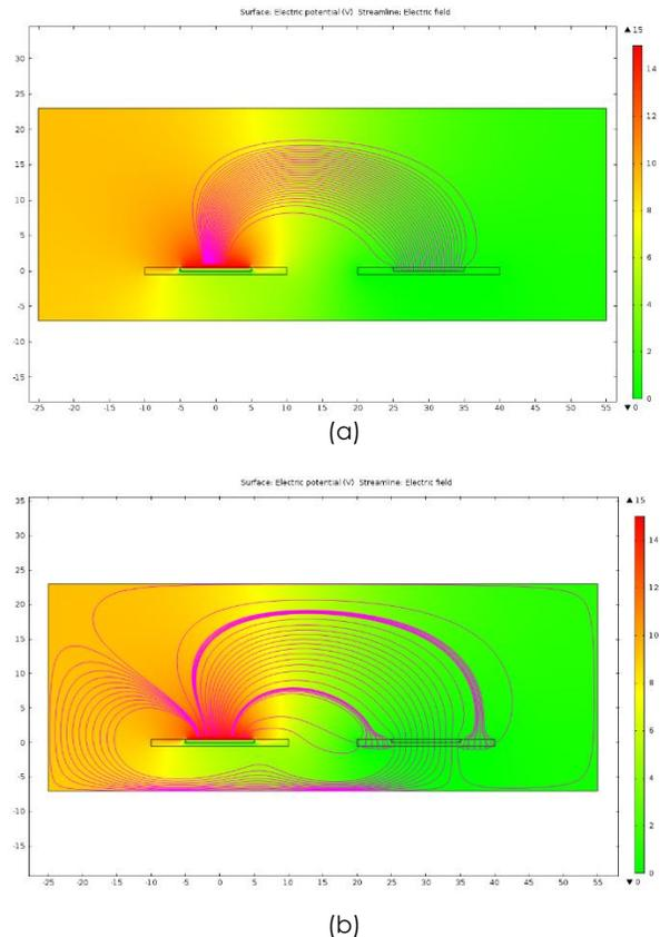
**Figure 7** FEM electric field streamline pattern (a) with driven guards and (b) without driven guards
