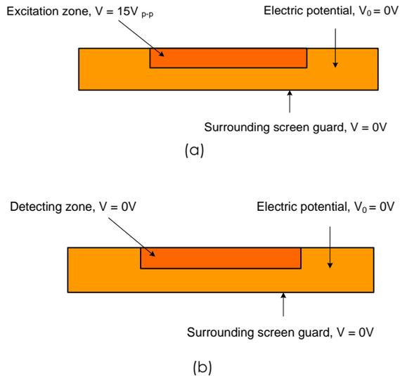
**Figure 5** Boundary conditions on (a) Excitation electrode and (b) detecting electrode
