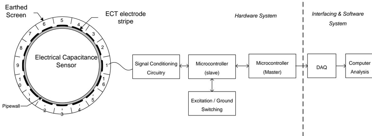
Figure 1 Electrical capacitance tomography system
