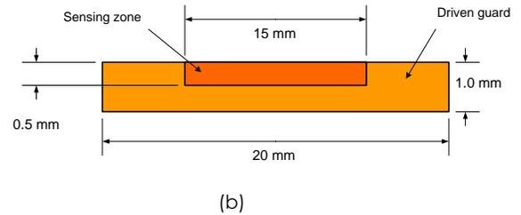
**Figure 4** ECT sensor geometry model for simulation; (a) two sensors in adjacent position inside an empty air (gas) space, (b) dimension of a single sensor in 2D
