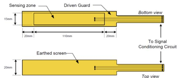
Figure 3 FR4 copper ECT sensor with embedded earthed screen and driven guard
