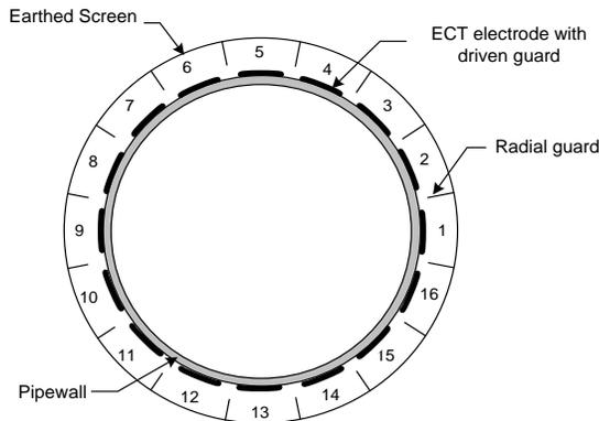
Figure 2 Cross-sectional view of ECT sensor design with guards
