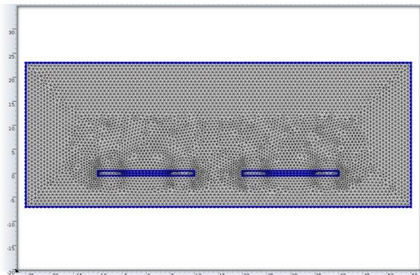
**Figure 6** Mesh size parameters with maximum and minimum element size of 0.8 mm and 0.0016 mm respectively
