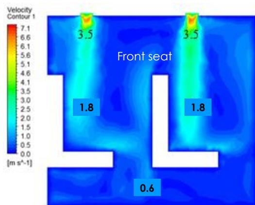
**Figure 9** The contour of air flow velocity distribution inside the passenger compartment for the displacement ventilation setup
