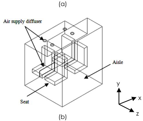
Figure 2 Simplified CFD model of quarter section of a bus passenger compartment. (a) Mixing ventilation setup and (b) Displacement ventilation setup
