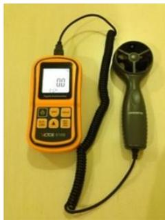
Figure 1 Digital anemometer
