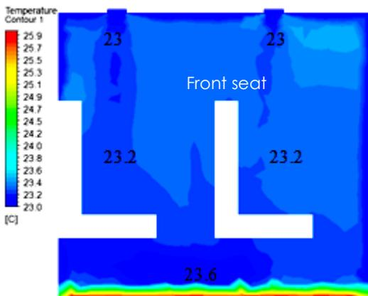
**Figure 7** The contour of air temperature distribution inside the passenger compartment for the displacement ventilation setup
