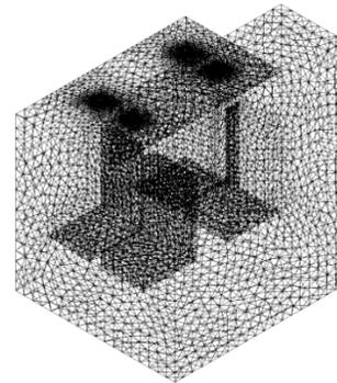
Figure 3 The meshed CFD model of the bus passenger compartment
