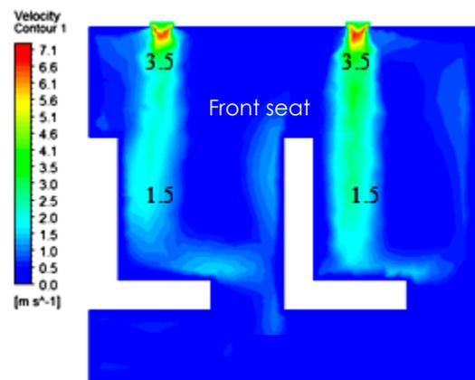
**Figure 8** The contour of air flow velocity distribution inside the passenger compartment for the mixing ventilation setup
