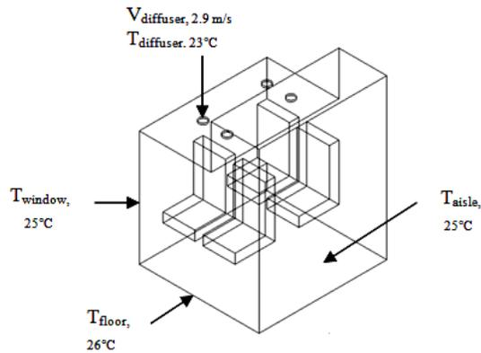
**Figure 4** The boundary conditions prescribed on the CFD model for turbulent flow analysis
