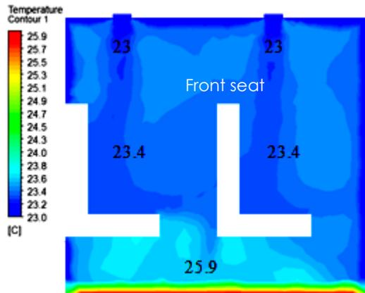
**Figure 6** The contour of air temperature distribution inside the passenger compartment for the mixing ventilation setup
