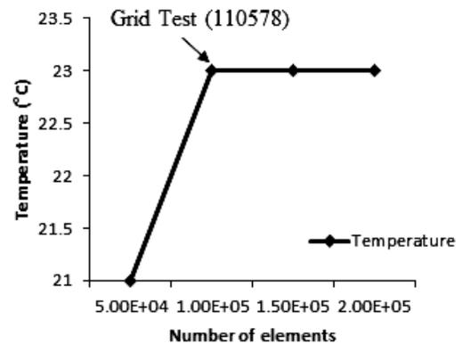
**Figure 5** Average air temperature versus number of elements used on the CFD model
