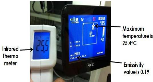
**Figure 3** Verification by comparing the emissivity value of 0.19 with infra-red thermometer
