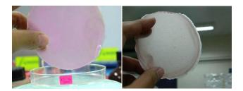
Figure 2 (a) Film from PSP and (b) Film from SP added with  $\ensuremath{\mathsf{BHA}}$
