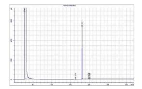
Figure 4 Methyl palmitate metyl ester standard chromatogram for gas chromatography analysis
