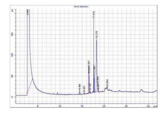
Figure 5 The chromatogram for the highest methyl palmitate methyl ester detection using gas chromatogram
