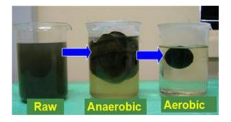
Figure 2 Treatment of raw textile wastewater using Microclear
