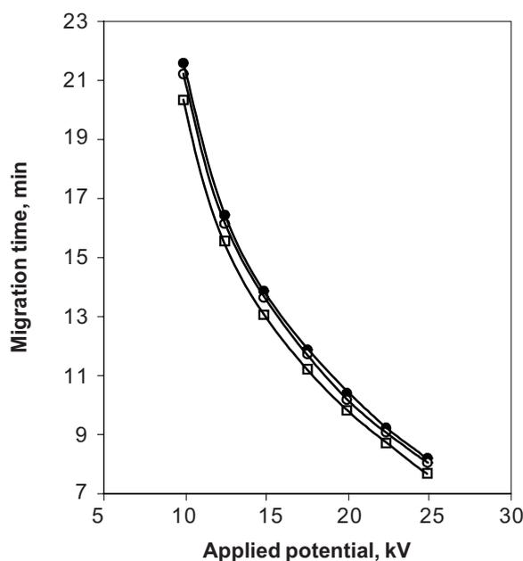
**Figure 4** Effects of applied potential on migration time of the batch 2 OPPs. Conditions: see Figure 2(b).  $\square$  phosphamidon,  $\circ$  dicrotophos,  $\bullet$  monocrotophos
