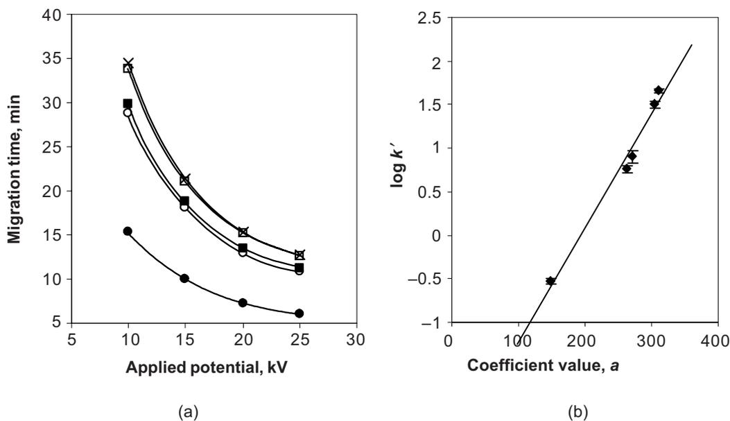
**Figure 3** (a) Effects of applied potentials on migration time of the batch 1 OPPs. Conditions as in Figure 2(a). Analyte identity: ● methidathion, ○ diazinon, ■ quinalphos, □ chlorpyrifos, × profenofos. (b) Relationship between the coefficient values of the regression lines against the log value of the capacity factors for the set of hydrophobic OPPs; error bars represent standard error
