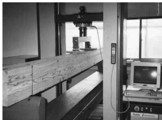
Figure 7 Full-scale four-point bending test setup
