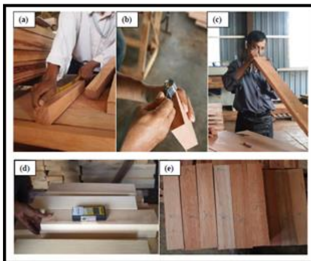
Figure 3 Visual grading process; a) measuring the specimen, b) identifying the species of the specimen, c) checking the defects, d) checking moisture content, e) grading the sample
