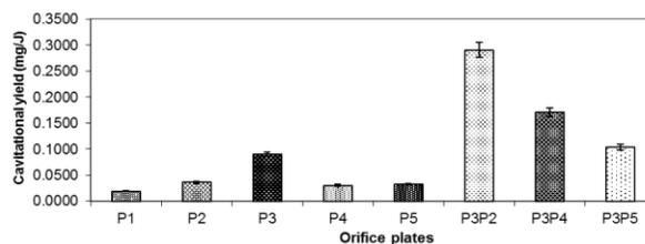
**Figure 6** Variation of cavitation yield for different plate configurations and plate arrangement
