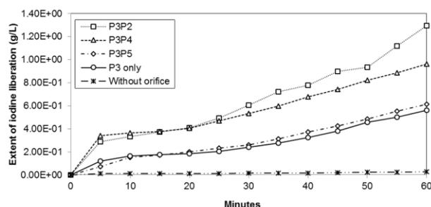
**Figure 5** Profile of iodine liberation for five different combination of plates
