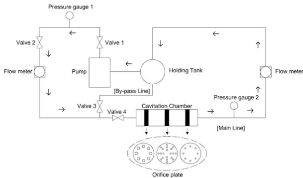
**Figure 2** Schematic diagram of hydrodynamic cavitation reactor setup
