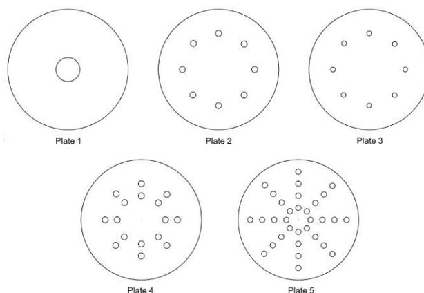
**Figure 1** Types of plate and arrangement of holes on the plates
