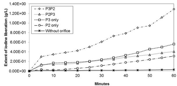
**Figure 4** Iodine liberation with different coordination of orifice plates
