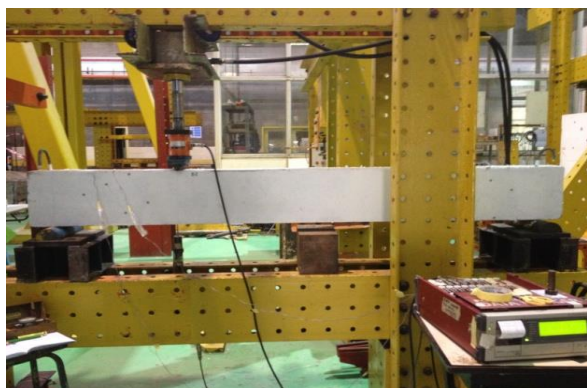
Figure 3 Test setup for shear test
