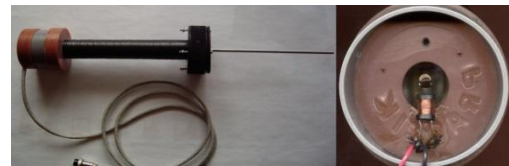
Figure 3 Resonance frequency sensor and its detail of drive coil on the right
