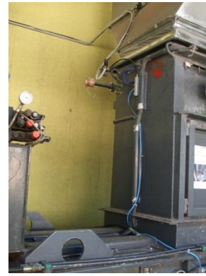
Figure 2 Chamber with the sensor that is mounted on its wall. The pieces of paper are transported through the chamber to the pressing machine for the pelleting process
