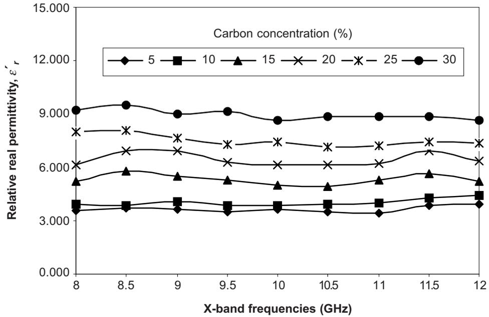
**Figure 6** Relative real permittivity,  $\epsilon'_r$ , at different carbon concentrations (%) in X-band frequencies (Pyrolysed carbon of 700°C)
