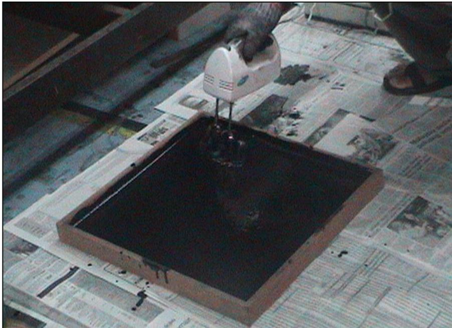
**Figure 2** Samples preparation using 450 × 450 mm wooden mould
