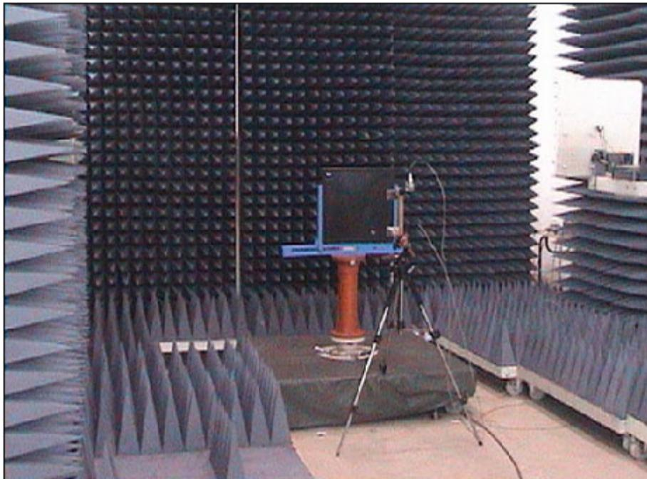
**Figure 3** Free space reflectivity measurement set-up
