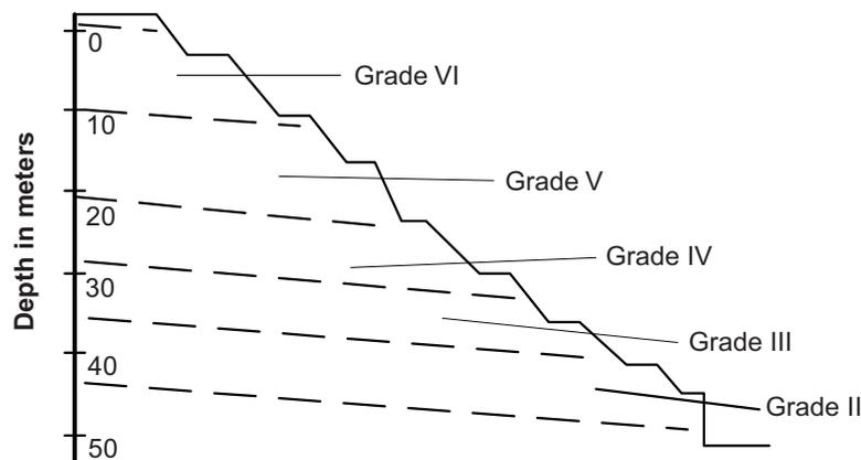
**Figure 1** Weathering profile of the cut slope at site A
