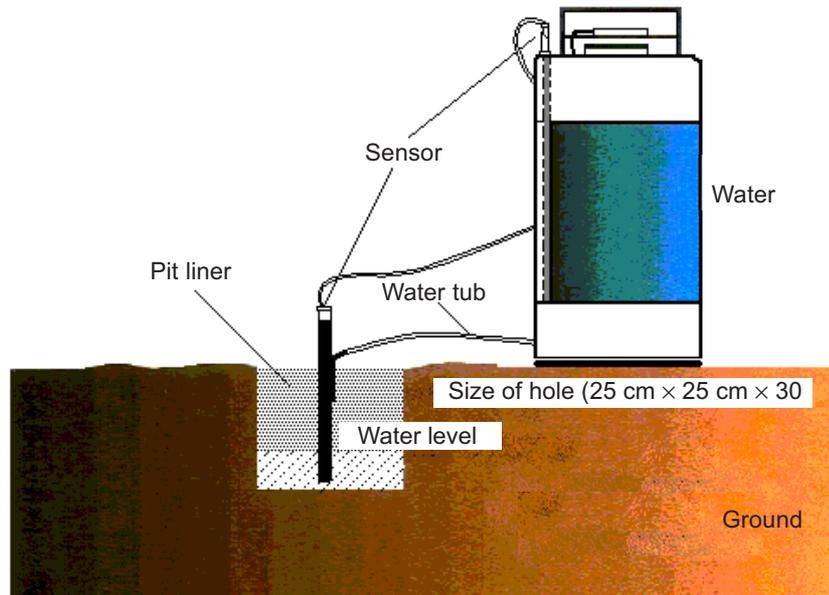
**Figure 3** Field infiltration test using Geonor infiltrometer
