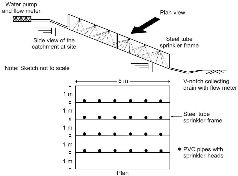
**Figure 5** Sprinkling frame and locations of sprinkler heads
