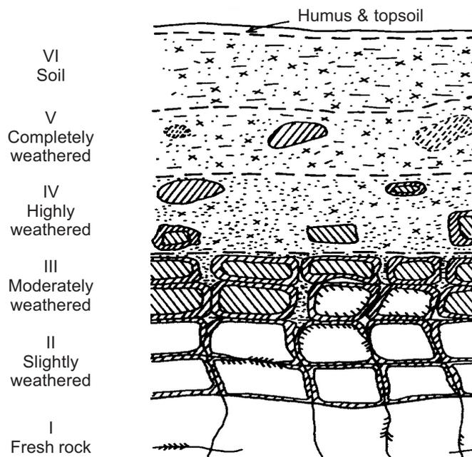
**Figure 2** Typical weathering profile in granitic rock (after Little [15])
