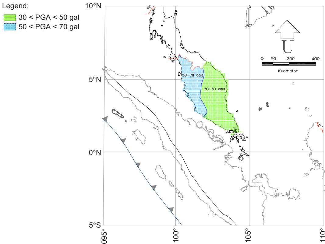
**Figure 11** PGA contour based on deterministic method
