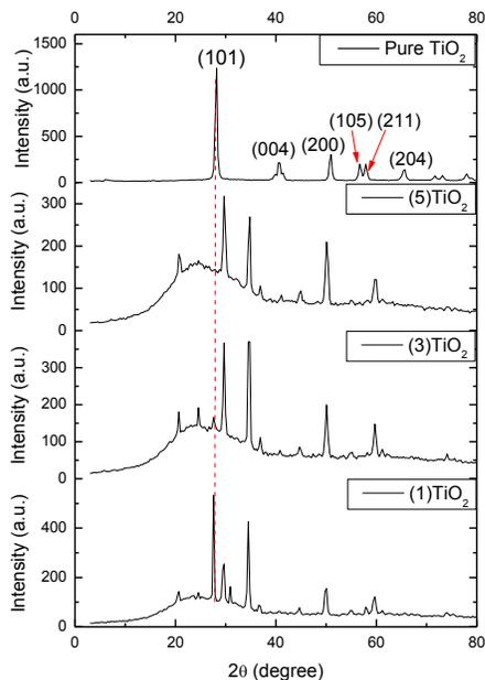
**Figure 4** The XRD pattern of TiO<sub>2</sub> NCs at different scan numbers
