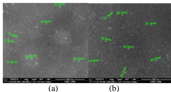
**Figure 3** The particle sizes of TiO<sub>2</sub> NCs at different scan number (a) (1) TiO<sub>2</sub> NCs (b) (5) TiO<sub>2</sub> NCs
