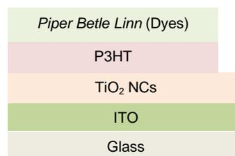
Figure 1 The schematic diagram of hybrid thin film
