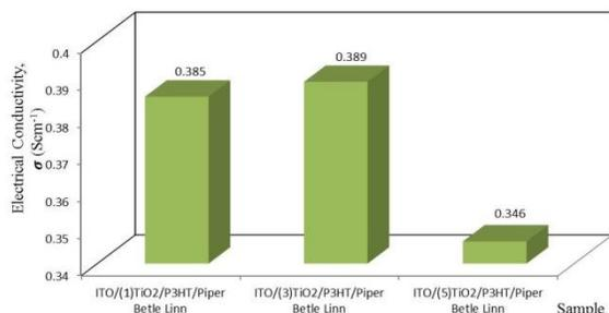
**Figure 5** The electrical conductivity of hybrid solar cell at different scan numbers of TiO<sub>2</sub> NCs
