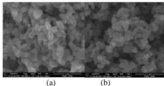
**Figure 2** The surface morphologies of TiO<sub>2</sub> NCs at different scan number (a) (1) TiO<sub>2</sub> NCs (b) (5) TiO<sub>2</sub> NCs
