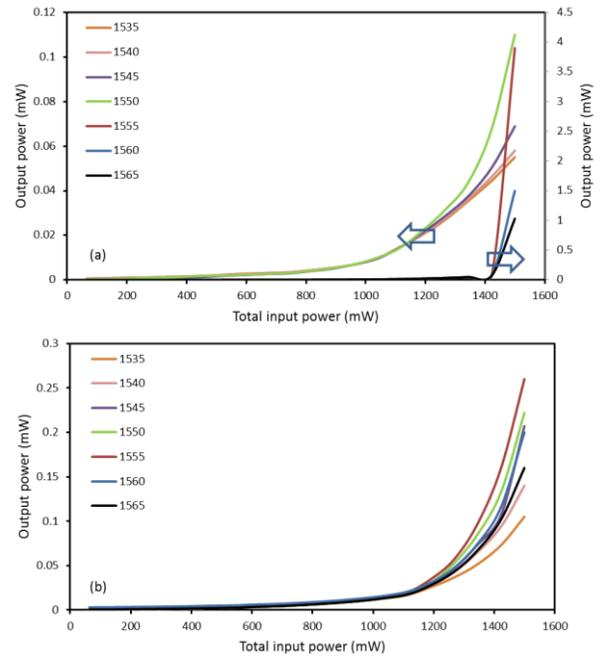
**Figure 2** Laser output for (a) outward and (b) inward pumping with varying pump power
