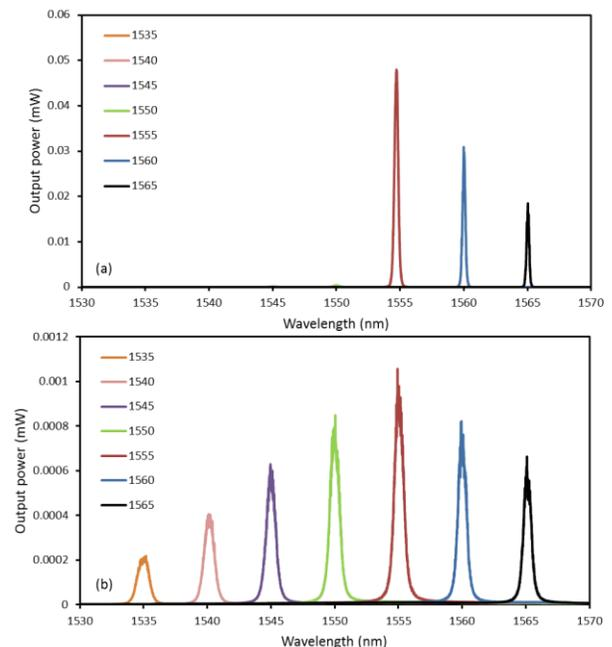
**Figure 4** Spectral output for (a) outward pumping and (b) inward pumping configuration at different wavelengths with maximum pumping power in linear scale
