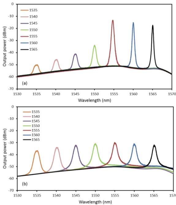
**Figure 3** Spectral output for (a) inward pumping and (b) outward pumping configuration at different wavelengths and at maximum pump power
