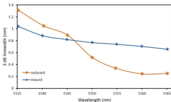
**Figure 5** 3 dB linewidth of the spectral output (every 5 nm in the range 1535-1565 nm) for outward pumping and inward pumping configuration
