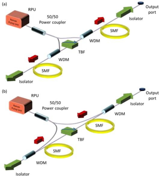
**Figure 1** Schematic of tunable RDB-FL employing (a) outward pumping and (b) inward pumping
