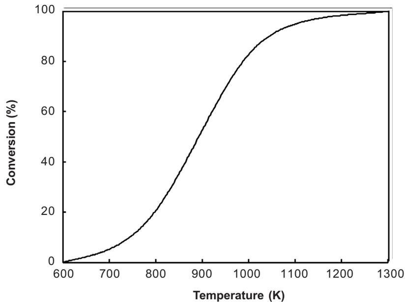
**Figure 1** Equilibrium reactant conversions for pure CORM reaction using MTE method
