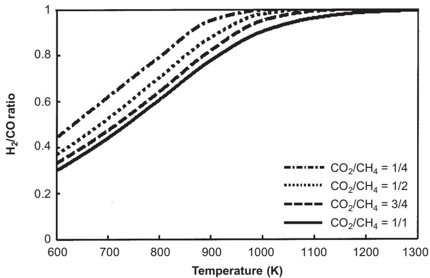
**Figure 7** Comparison of H<sub>2</sub>/CO ratios as a function of temperature with different CO<sub>2</sub>/CH<sub>4</sub> ratios using LUM method
