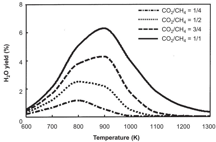
**Figure 6** Comparison of water yields as a function of temperature with different CO<sub>2</sub>/CH<sub>4</sub> ratios using LUM method
