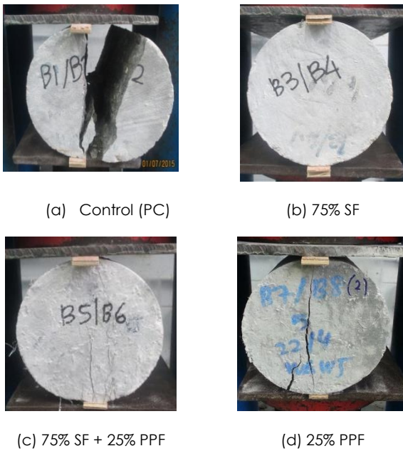
Figure 7 Failure mode of the cylindrical specimens
