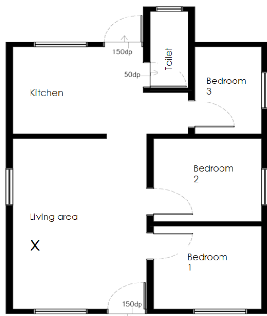
Figure 3 (a) PPRT modern concrete house in Kampung Batu 16, Gombak, (b) exposed roof structure in H2 and (c) its floor layout, 'X' marks the location of OHM Delta Instrument
