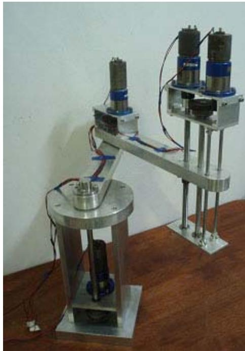
**Figure 13** Overview of the 4-DOF SCARA robot
