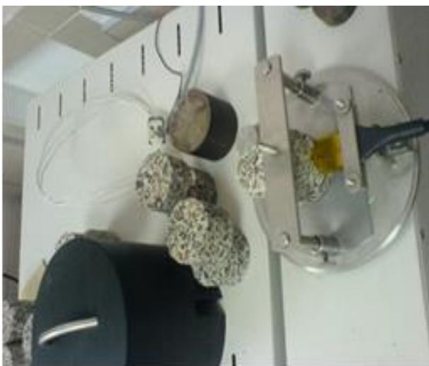
Figure 1 Set-up of Hot disk thermal constant analyzer for thermal test with a Hot-Disk probe TPS2500
