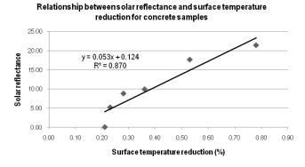
Figure 6 Regression of solar reflectance and surface temperature reduction of concrete sample
