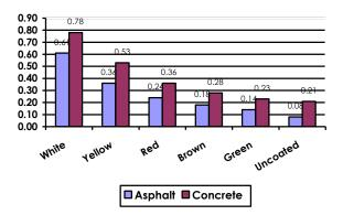
Figure 2 The solar reflectance of the tested color coated and uncoated for asphalt and concrete samples
