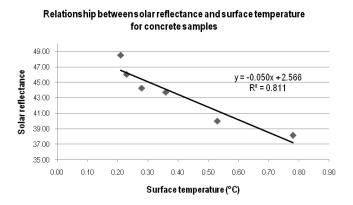
Figure 5 Regression of solar reflectance and surface temperature of concrete sample
