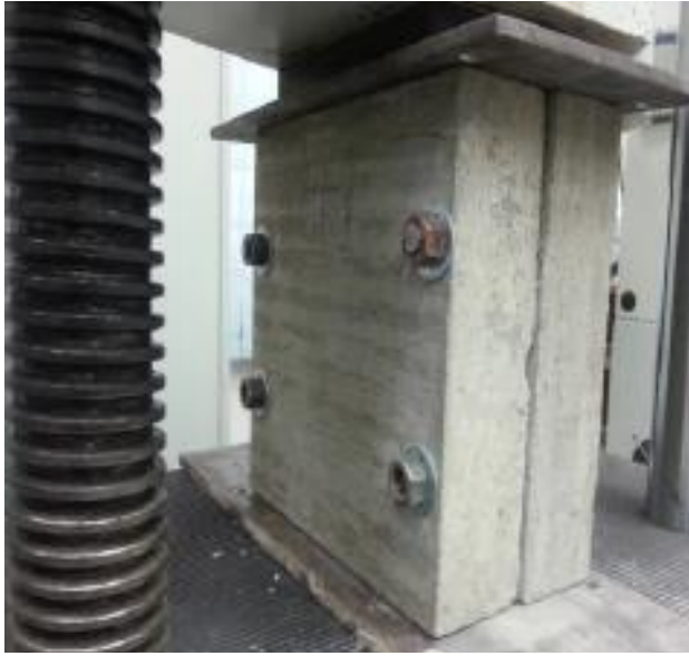
Figure 4 Compression test of prototype of LFC wall panel
