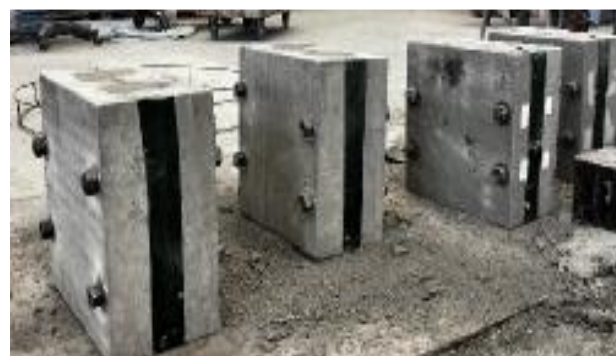
Figure 3 Prototypes of LFC wall panel after curing process
