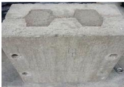
Figure 16 The sample without any mechanical connectors
