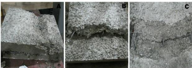
**Figure 3** Failure of OPSPAC wall panel specimens (R-32, P-32, P-34)
