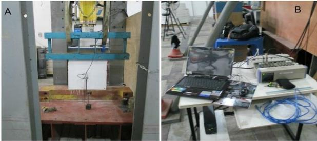
**Figure 2** (A) OPSPAC wall panel set-up for compression test; (B) Data logger
