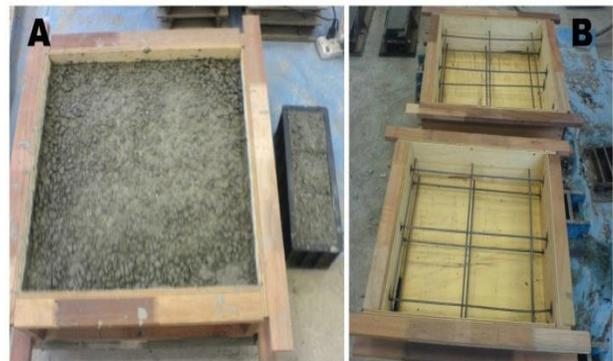
**Figure 1** (A) Specimens cast in a horizontal formwork; (B) Formwork with two layers of BRC A6
