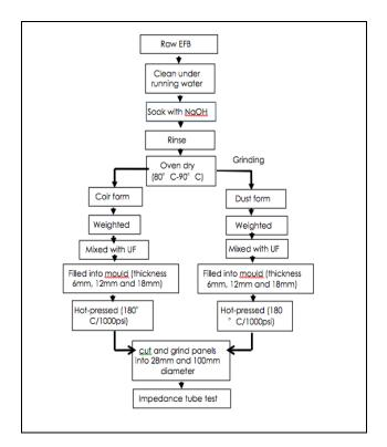
Figure 1 Process Chart for Sample Preparation
