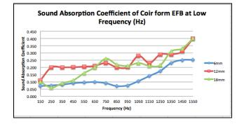
Figure 4 Sound absorption coefficient of coir form EFB at low frequency region
