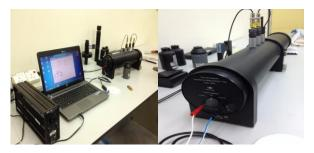
Figure 2 Impedance tubes
