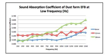
Figure 3 Sound absorption coefficient of dust form EFB at low frequency region
