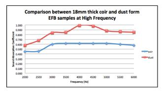
Figure 8 Sound absorption coefficients of 18mm thick coir and dust form EFB at high frequency region
