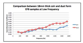
Figure 7 Sound absorption coefficients of 18mm thick coir and dust form EFB at low frequency region
