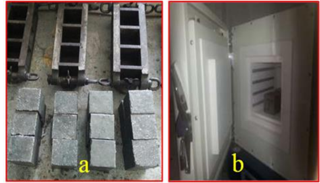
Figure 1 Curing method (a) ambient curing (b) oven curing
