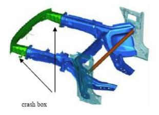
Figure 1 Crash box placement on chassis [6]
