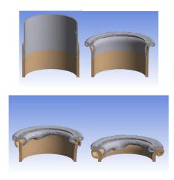
Figure 6 Deformation sequence of two segments crash box
