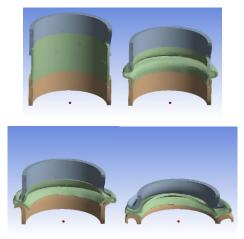
Figure 8 Deformation sequence of three segments crash box (type 2)
