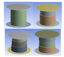
Figure 2 Crash box model: 1 segment, 2 segments, 3 segments (type 1) and 3 segments (type 2)
