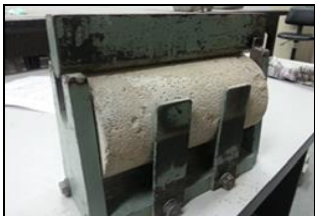
Figure 8 Setup of a cylindrical shaped specimen for tensile strength test
