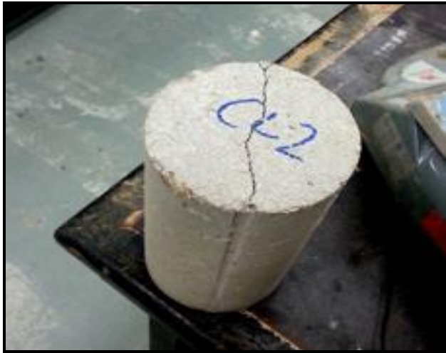
(a) Cracks formed on sample CF-0.4
