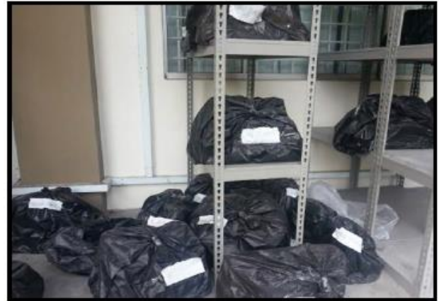
Figure 8 Sealed curing condition of foamed mortar samples in the lab
