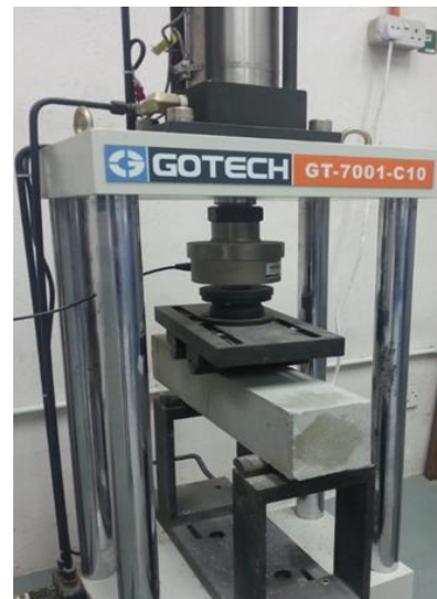
Figure 1 Sample being tested by the compressive machine
