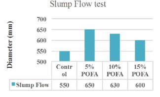
Figure 1 The bar graph of Slump Flow Result
