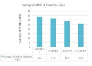
Figure 5 Results of Modulus of Elasticity
