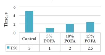
T500 Slump Flow Test
