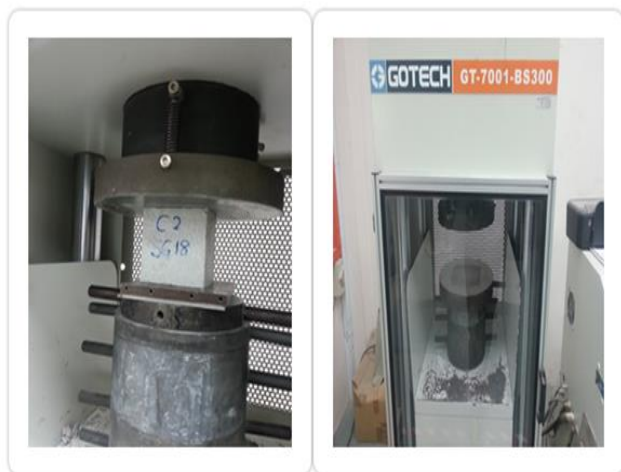
Figure 1 Sample being tested by the compressive machine
