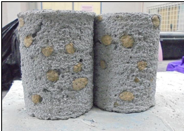
Figure 2 Cylinder shape lightweight aggregate foamed concrete obtained from the prism
