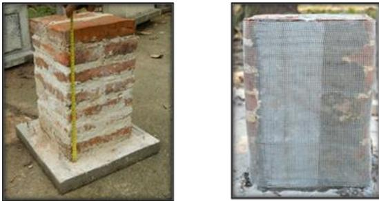
Figure 3 Masonry prisms for test
