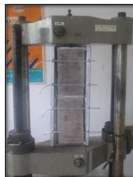
**Figure 2** Shear bond testing
