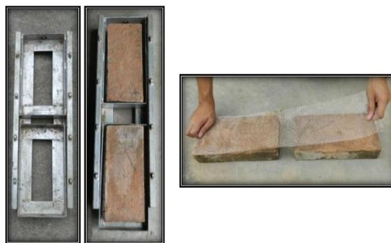
**Figure 1** Special designed steel device for testing
