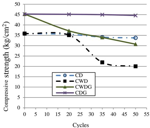
**Figure 7** Compressive strength of strengthened or un-strengthened specimens under wet-dry cycles
