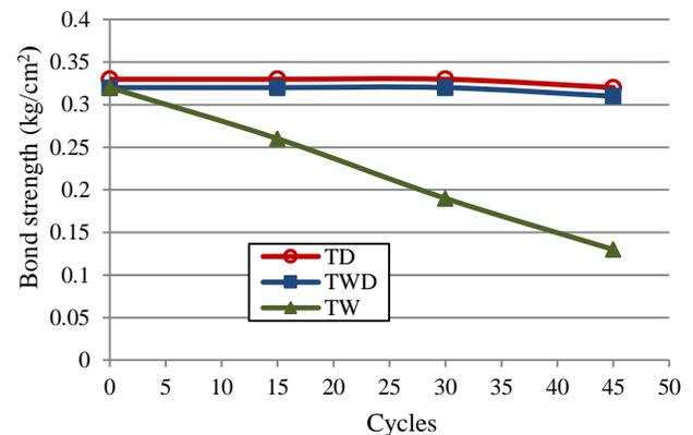
Figure 5 Change of bond strength in different conditioning
