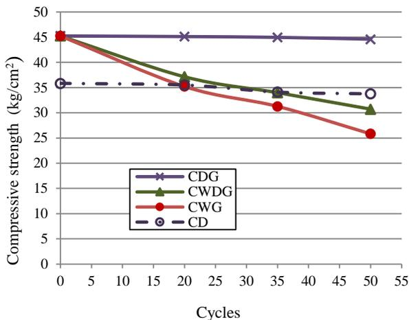
**Figure 6** Strength degradation of GFRP strengthened prisms exposed to different conditions
