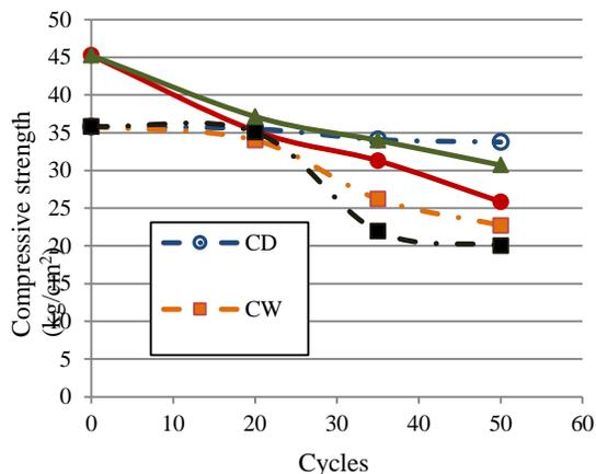
**Figure 8** Compressive strength under Long-term moisture environment or wet-dry cycles
