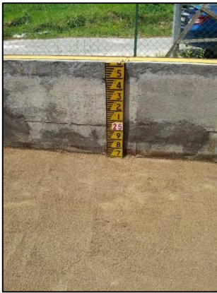
Figure 4 Stick levelling gauge attached to the inner side wall of river model
