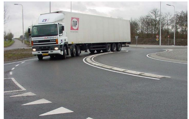
Figure 8 Traversing of lane divider by a semitrailer [3]
