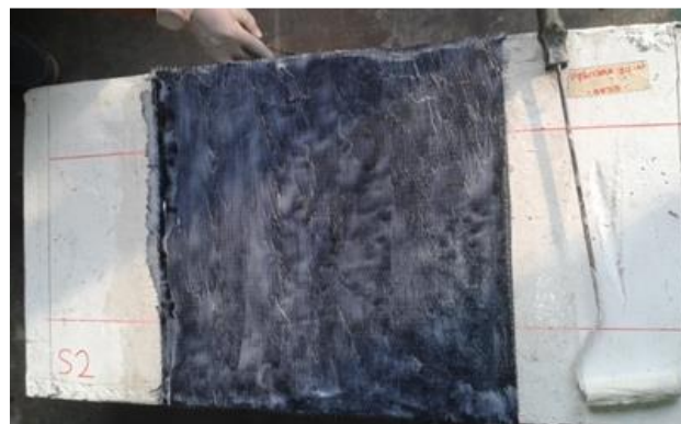
Figure 2 Epoxy bond covered on the top of slab 2
