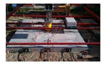
Figure 2 The complete assembly for static load test
