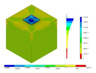
**Figure 7** Distribution of normal stress  $\sigma_z$ , vertical section through the subsoil model [Pa]
