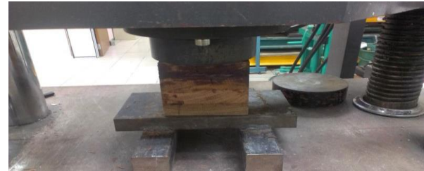
Figure 5 Testing specimen using Universal Testing Machine (UTM 1000)
